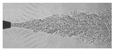
laminar helium jet into air (0.26 cm nozzle) 85kHz weak shock wave along 60° cone from Chan & Lee (1972)
