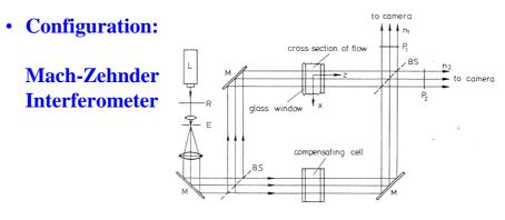
• If density variation are present, then phase differences between the object path and reference path result, which lead to interference patterns after
