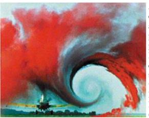
Aircraft wake vortices can throw treacherous air turbulence into the paths of succeeding planes. In this NASA/FAA test, colored smoke makes the swirling airflow visible. NASA LANGLEY RESEARCH CENTER (from SCIAM 2002/02)
